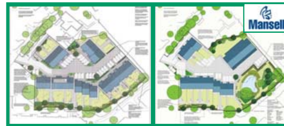
Conservation gains: as a result of ecological surveys, a housing plan was redesigned to retain the pond and wetland feature.
